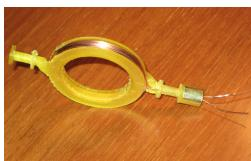
about 5cm from the end. Then start winding the wire around the armature frame, this is made easy by the sides of the frame being open at each end. Once the wire windings are flush to the edge of the plastic frame cut the wire generously and feed back though the hollow shaft alongside the first wire.
