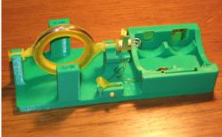
Before installing the armature into the base it will be necessary to put a little bit of inward preload onto the brushes, this will keep them in
