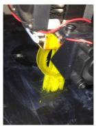
For simplicity the armature frame is combined with the bearing shafts and commutator as a single piece. The armature should be printed vertically with 100% infill, supports turned on everywhere and set to a high print quality. The switch can also be printed at the same time.
