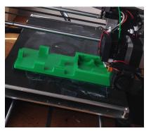
Once the base has finished printing the grooves will require cleaning out with a fine blade, the horizontal brush holder grooves will need the most attention. The armature will need the supports trimmed off with a sharp hobby knife and the bearing surfaces smoothed out with a file or fine sandpaper.
